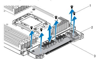
Figure 3-17. Removing and Installing the Interposer Extender
